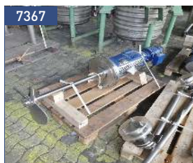
propeller mixer, 316 (1.4571) 0,75 kW - 123 rpm
