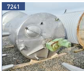
volume 8 cbm, 304 insulation 2,2 kW - 42 rpm
