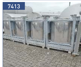
volume 1 cbm, 304 - round container - outside high-gloss frame Fe (galvanized)
