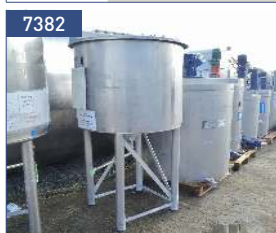
volume 1 cbm, 304 0,75 kW - 104 rpm yoc.: 2009
