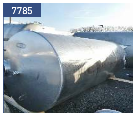
volume 12 cbm, 316 (1.4404) lateral agitator flange
