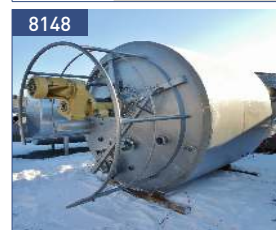
volume 11,2 cbm, 316 (1.4571) wt.: 3/4 mm insulation agitator: 7,5 kW - 36 rpm drawing
