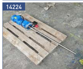
agitator, 316 (1.4571) - brand new - 1,5 kW - 270 rpm without propeller
