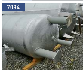
volume 8 cbm, 304 wt.: 5 mm 9,9/16 kW - 45/90 rpm TÜV-certificates
