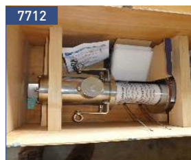
pneumatic-agitator, 316 (1.4401) - unused - 0,75 kW - 2885 rpm
