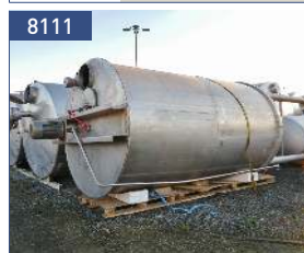
volume 12 cbm, 304 double jacket (304) lower bottom propeller 1,5/7,5 kW-480/970 rpm
