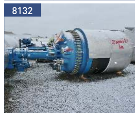
volume 8,2 cbm, Fe (enamelled) inside: -1/+6 bar double jacket, Fe: -1/+7 bar insulation anchor stirrer
