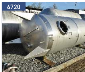
volume 8,2 cbm, 304 heating coils inside magnetic stirrer 1,1 kW - 910 rpm
