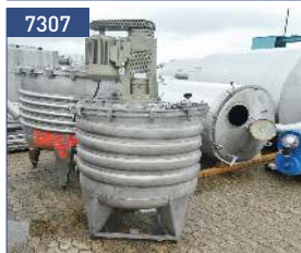
volume 1 cbm, 304 inside: 0,5 bar half-coils, 304: 1 bar anchor: 1,5/4,5 kW
