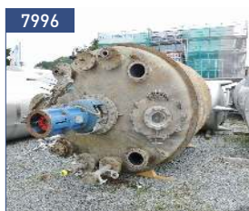
volume 13,3 cbm, 316 (1.4571) inside: -1/+6 bar half-coils, 316: -1/+6 bar test certificates
