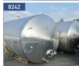
volume 12 cbm, 316 (1.4401) bearing shells Fe (lacquered)
