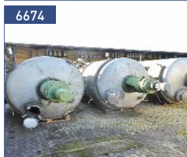
volume 12,5 cbm, 304 (1.4541) double jacket, Fe special anchor 2 kW - 7 rpm
