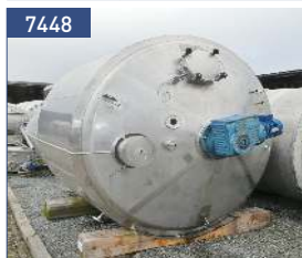
volume 8 cbm, 304 inside: 0,4 bar insulation anchor: 4 kW - 16 rpm
