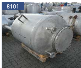
volume 1 cbm, 316 (1.4571) -1/+6 bar wt.: 6/8 mm TÜV-certificates
