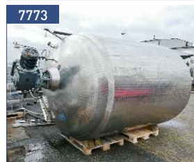
volume 8 cbm, 304 half-coils, 304 insulation agitator: 4 kW - 14 rpm
