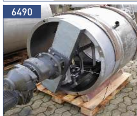
volume 1 cbm, 304 anchor with plastic scrapers 2,2 kW / 4,5 - 34 rpm
