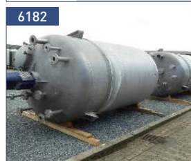
volume 8 cbm, 304 [1.4541] blades stirrer 22 kW - 61 rpm order no. 6182
