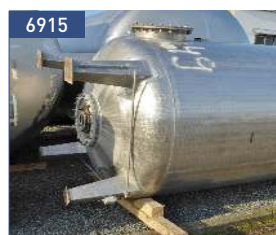
volume 9 cbm, 304 7,5 kW / 20 - 125 rpm
