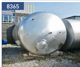
volume 12 cbm, 304 (1.4541) 3,5 bar; wt.: 4/8 mm double jacket, lower bottom, 304 TÜV-certificates
