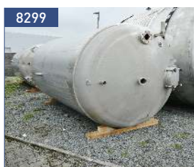
volume 9 cbm, 304 inside: -1/+3,5 bar doublejacket, 304 with trickle ring documentation
