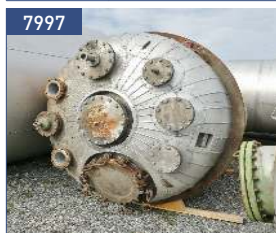
volume 8,6 cbm, 316 [1.4571] inside: -1/+6 bar half-coils, 304 [1.4541]: -1/+20 bar insulation, Fe-jacket (galvanized; upper bottom)
