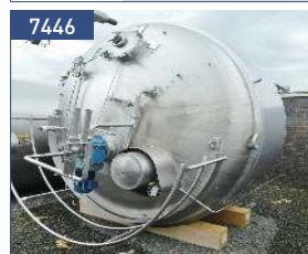
volume 11,7 cbm, 316 (1.4401) inside: 0,99 bar double jacket with drip ring agitator: 1,2/2,2 kW - 12/25 rpm
