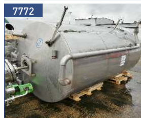
volume 8 cbm, 304 blades stirrer without motor/gear
