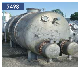
volume 13 cbm, 316 (1.4404) -1/+3 bar; wt.: 6/7/9 mm heating bundle, 316: -1/+6 bar TÜV-certificates
