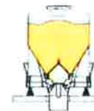
IBC lowered and station raised
