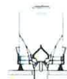
IBC empty, cone valve product discharge
